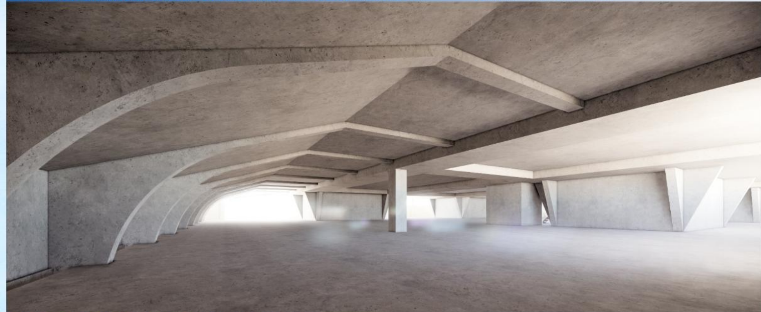
3D MODEL: DESIGN OF BASEMENT FLOOR STRUCTURE
