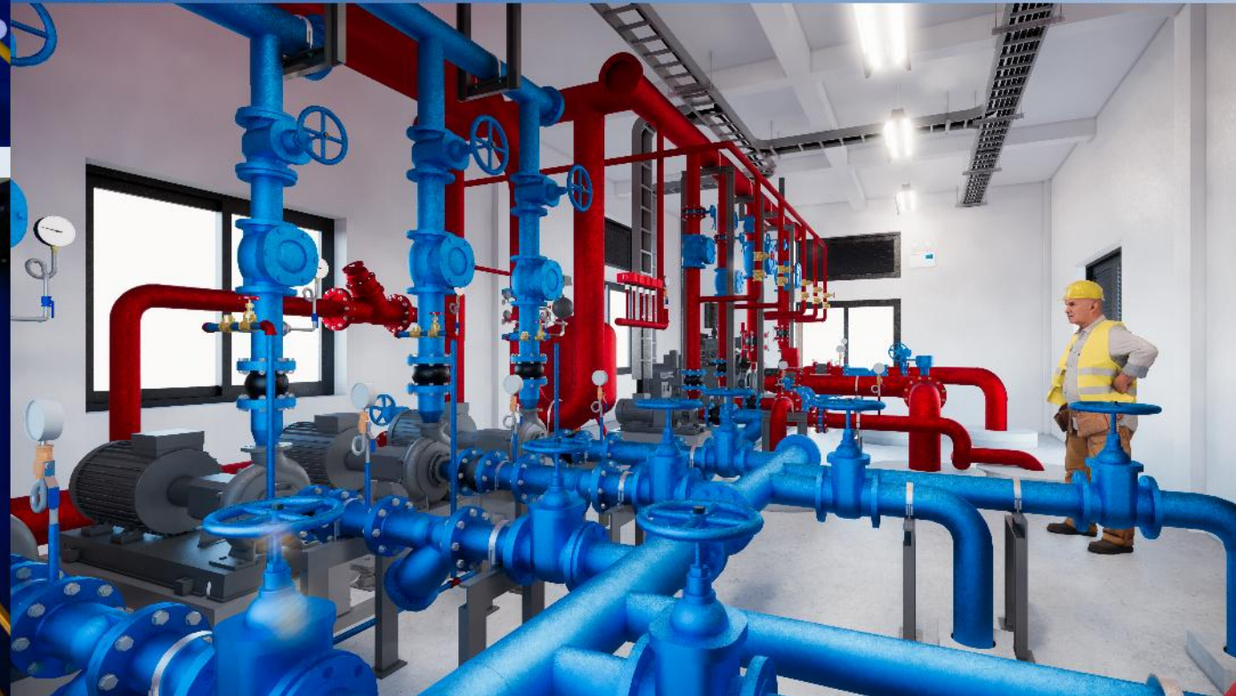
3D MODEL: DESIGN OF FIREFIGHTING PUMP SYSTEM
