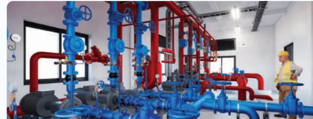
3D Model: Design of Firefighting Pump System
